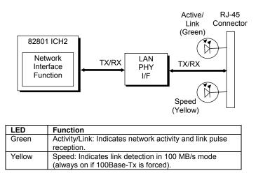
Figure 5-13. Network Interface Controller Block Diagram
